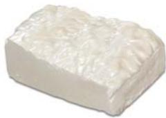
ThermalGuard OC1 is an open cell, 100% water-blown spray polyurethane foam insulation system with a density of 1.0 lb and an R-value of 4.7 per inch. When applied, ThermalGuard OC1 expands to over 50 times in size in approximately 8 seconds, filling and sealing building cavities of any shape and size. It achieves twice the yield of 2.0 lb spray foam while reducing waste and cleanup time by up to 50% compared to that of a ½ lb spray foam insulation.
